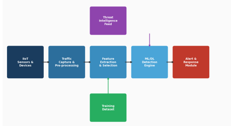
Fig. 3. IDS Framework Data Flow and Component Interaction for IIoT Networks
