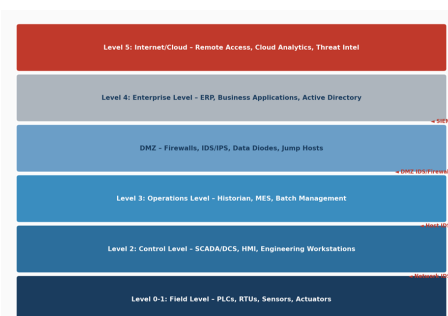
Fig. 2. Purdue Reference Model Adapted for Proposed IIoT Security Architecture with IDS Placement
